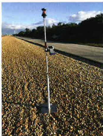
Figure 7: Monitoring the elevations. 12" square aluminum plate fixed to the bottom of a survey rod to allow for a measurement of the top of the crawlerway road surface, ensuring the rod tip did not fall between individual rocks (left). Bespoke mount for level rod to monitor ground at an instrument setup within the CT zone of influence (center). Monitoring the ground at an instrument location outside the CT zone of influence (right).
