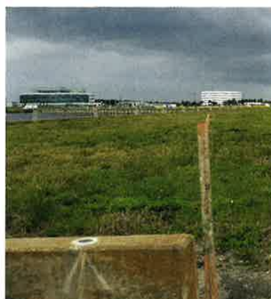
Figure 5: Vertical control survey: a closed digital level loop was used to establish elevations for all control points set (left). Control level run started from an NGS monument near the VAB (center and right).
