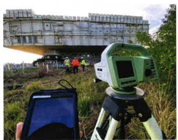
Figure 7: Monitoring the elevations. 12" square aluminum plate fixed to the bottom of a survey rod to allow for a measurement of the top of the crawlerway road surface, ensuring the rod tip did not fall between individual rocks (left). Bespoke mount for level rod to monitor ground at an instrument setup within the CT zone of influence (center). Monitoring the ground at an instrument location outside the CT zone of influence (right).
