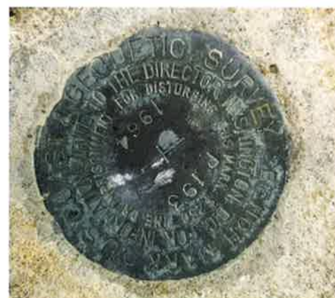
Figure 5: Vertical control survey: a closed digital level loop was used to establish elevations for all control points set (left). Control level run started from an NGS monument near the VAB (center and right).
