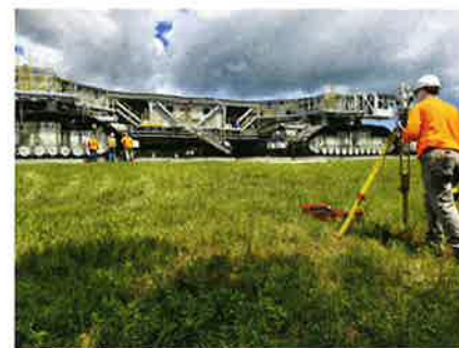
Figure 4: Finished bracket mounted to the CT truck (left)— 2" square tubing 11 feet long, 4 feet high, supported with 3/4" steel tubing, all attached without damaging or altering the surface of the CT. Measuring the height of prism relative to the crawlerway road underneath the CT trucks (center). Testing prism bracket and potential monitoring procedures during a planned move of the CT (right).
