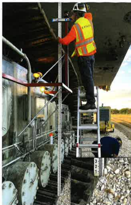
Figure 4: Finished bracket mounted to the CT truck (left)— 2" square tubing 11 feet long, 4 feet high, supported with 3/4" steel tubing, all attached without damaging or altering the surface of the CT. Measuring the height of prism relative to the crawlerway road underneath the CT trucks (center). Testing prism bracket and potential monitoring procedures during a planned move of the CT (right).
