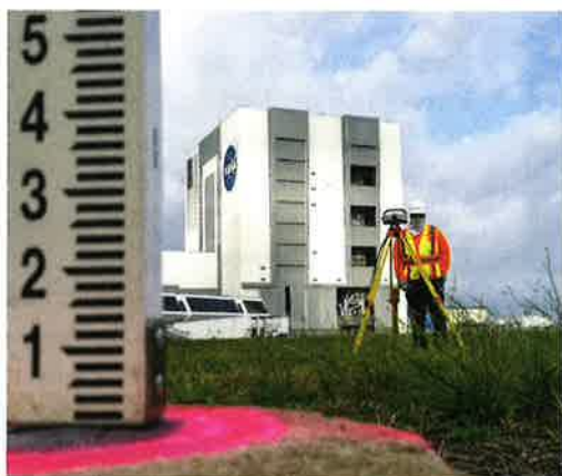
Figure 5: Vertical control survey: a closed digital level loop was used to establish elevations for all control points set (left). Control level run started from an NGS monument near the VAB (center and right).
