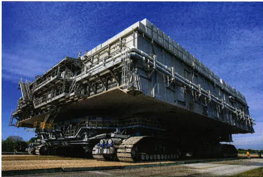
Figure 1: CT fully loaded with concrete blocks. Total weight for this pass was 25 million pounds.
