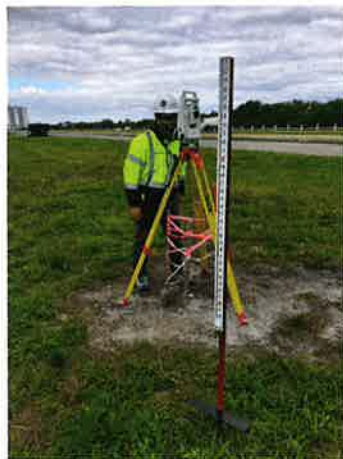
Figure 7: Monitoring the elevations. 12" square aluminum plate fixed to the bottom of a survey rod to allow for a measurement of the top of the crawlerway road surface, ensuring the rod tip did not fall between individual rocks (left). Bespoke mount for level rod to monitor ground at an instrument setup within the CT zone of influence (center). Monitoring the ground at an instrument location outside the CT zone of influence (right).
